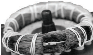
Fig. 44 PTC sensor incorporated in windings
