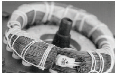
Fig. 46 Thermal switch incorporated in windings
