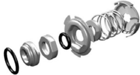
Fig. 6 Exploded view of shaft seal
