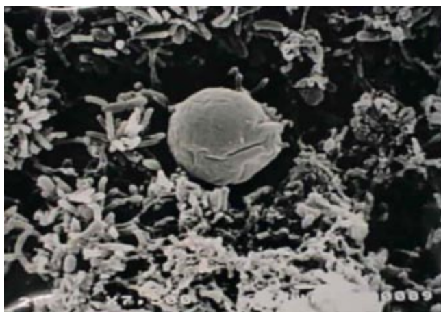
Figure 3 — SEM of biofouled membrane. Magnification x7,500.
