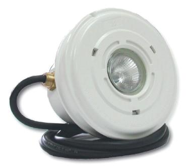
The IM 3700 is manufactured from ABS plastic and is equipped with an aluminum reflector and a borosilicate lens for high light quality. It has a standard MR16 type 50W Halogen lamp.
