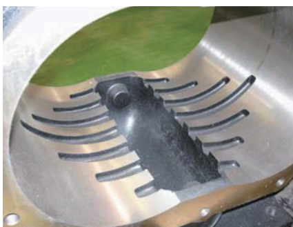
Pulse eraser (pressure pulsation reduction mechanism)
