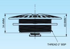
Material: High strength ABS. Maximum Operating Temperature: 50°
