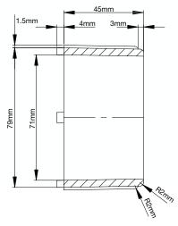
Material: High strength ABS. Maximum Operating Temperature: 50°
